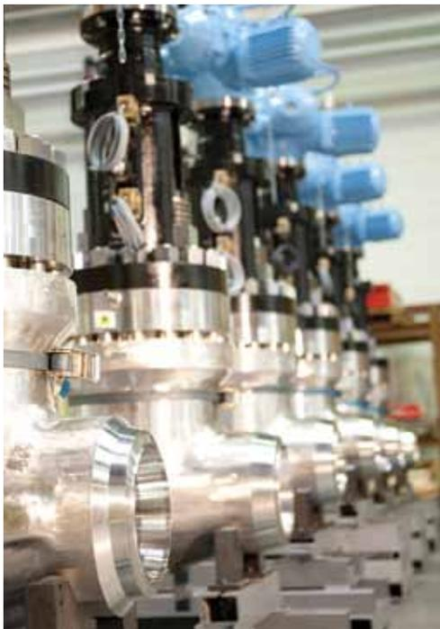
*Large forged gate valves lined up for Taishan.*
