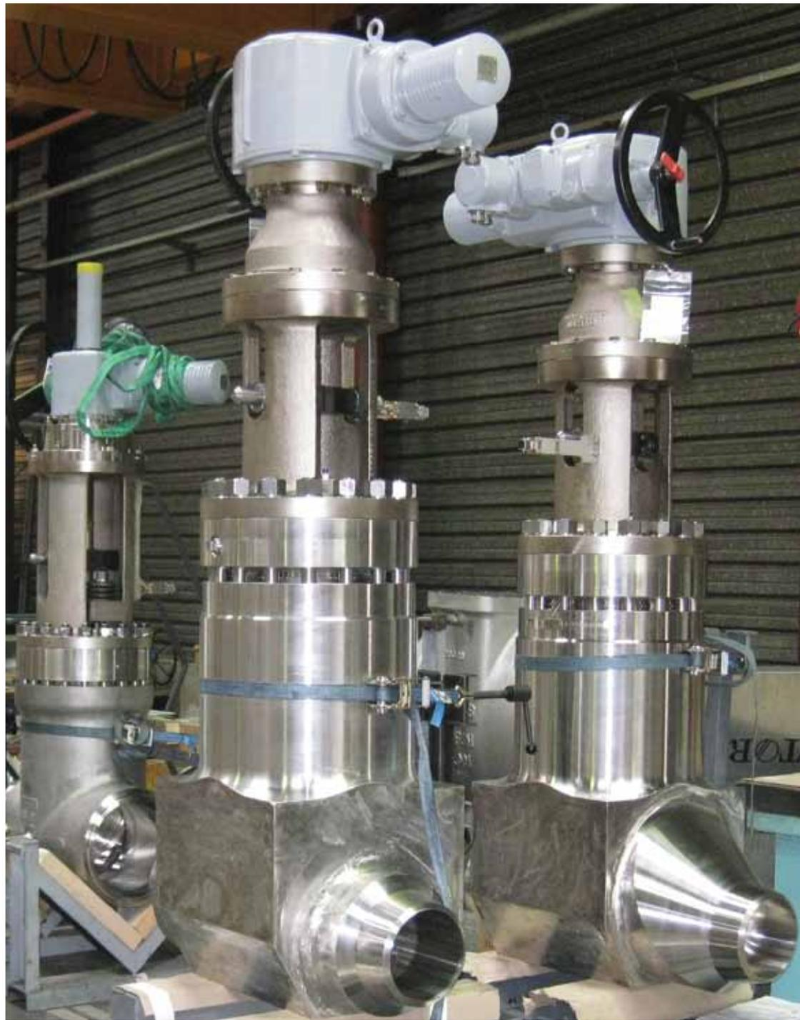
*Large-size bellows seal valves ready to be shipped to the Taishan EPR™ site.*
