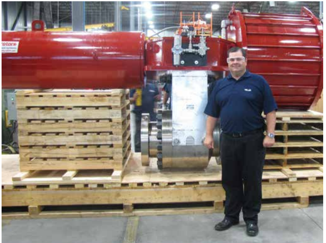
Paul Dion, Velan's VP of Sales, Canada, stands beside a 16" metal-seated ball valve complete with a 22' Rotork actuator, the largest actuator built by the company. The valve is ready for shipment to Meridian and is intended for use in a SAGD application in northern Alberta, Canada.
