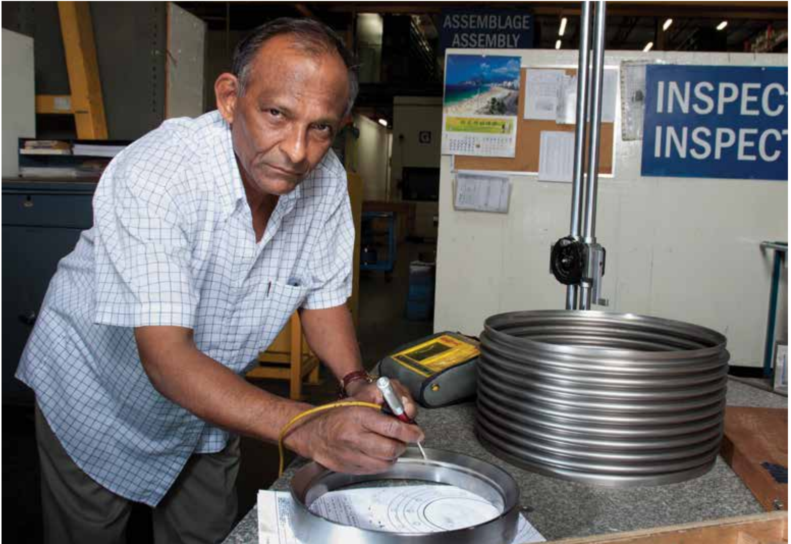
Chiman performing measurement testing on the seat that will be installed within a metal-seated ball valve.
