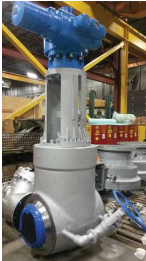
A 20” pressure seal, 2900 special class gate valve with an electric actuator, is prepared for a shipment of valves destined for India.
