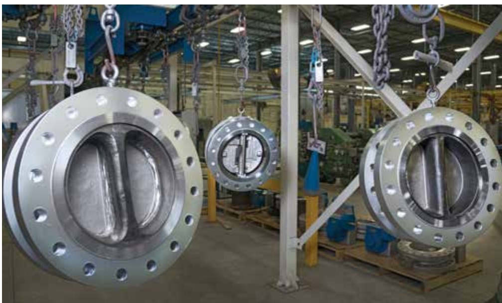
Velan Proquip dual-plate check valves in production.
