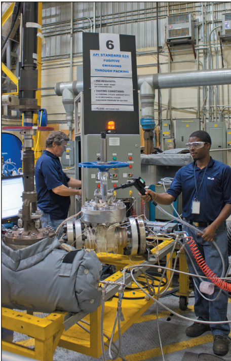
API 624 fugitive emissions qualification testing.
