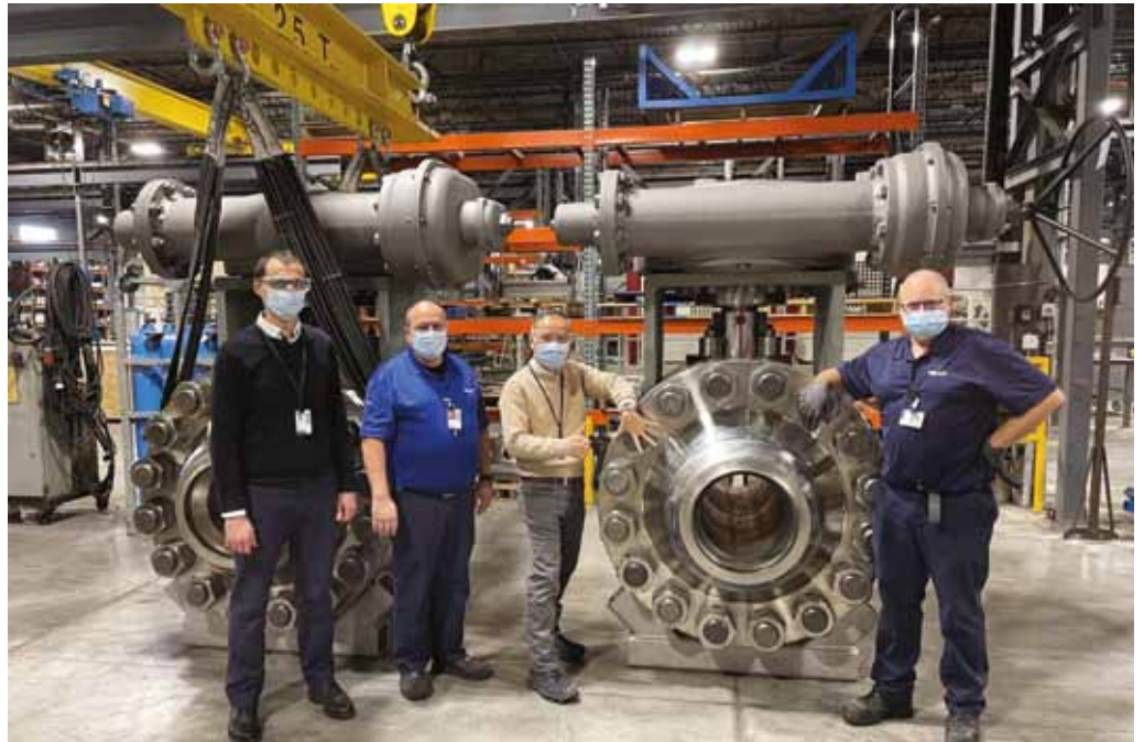
Velan high performance ANSI-2500 isolation valves for residue hydrocracking
