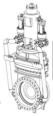
Custom designed NPS 30 (DN 750) stainless steel gate valve with two forged NPS 4 (DN 100) bypass valves, completely controlled by 40' reach rod system
