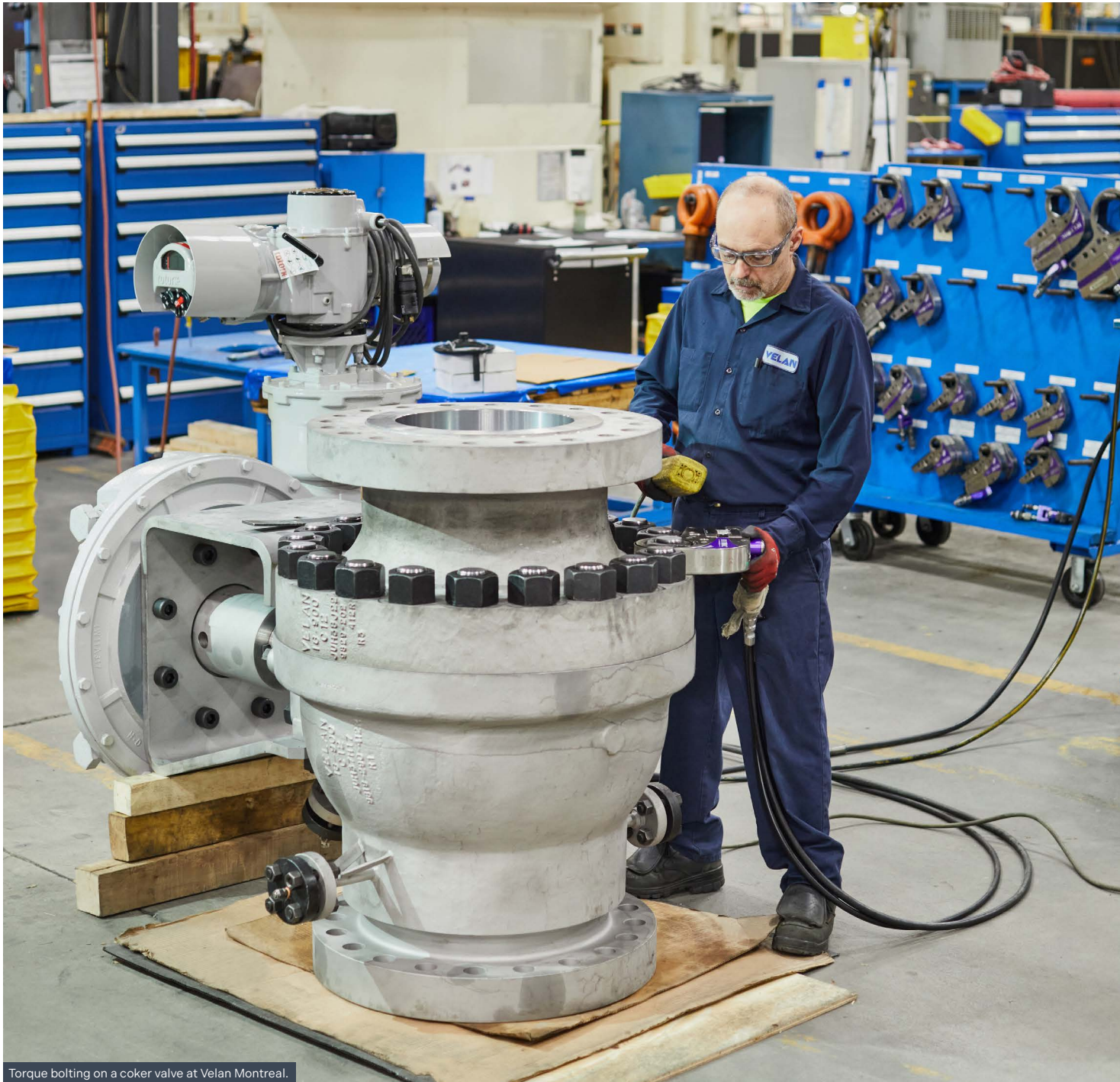
Torque bolting on a coker valve at Velan Montreal.
