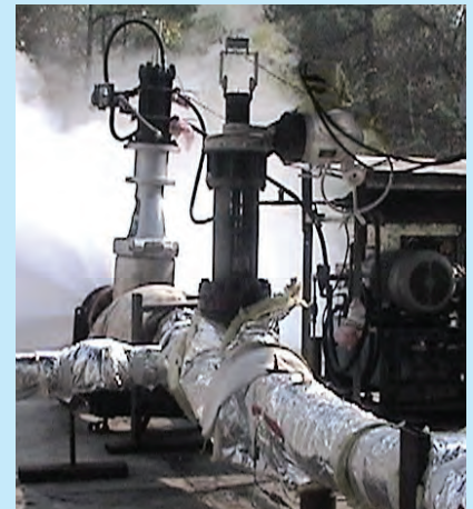
Loop isolation valve blowdown test with hot pressurized water of Velan electrically actuated NPS 8 (DN 200) class 900 regular port loop isolation valve. The water flashes to steam in a starburst pattern as it blows down to atmosphere.
