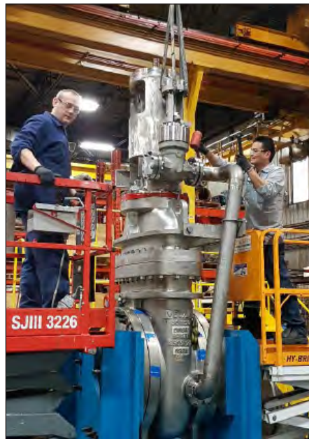
Custom made hydro-testing rig designed for testing larger valves in-house.
