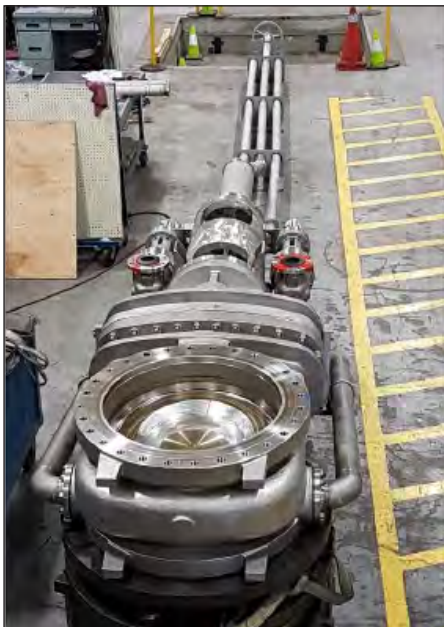
NPS 30 (DN 750) gate valve displaying 40' reach rod system.
