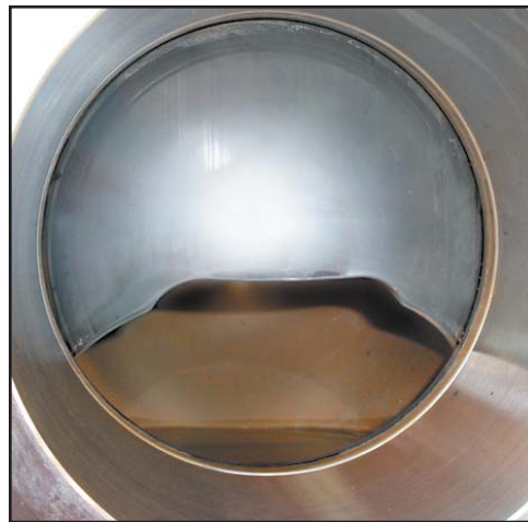
Ball with ceramic coating in half open position, after several months in service.
