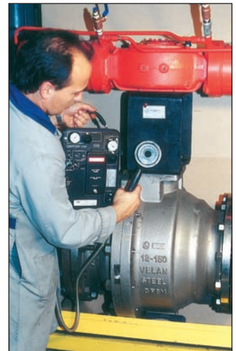
Velan performs emissions testing to guarantee our valves meet strict low emission criteria.
