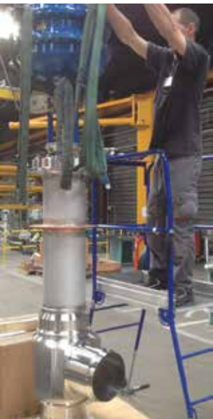
Angle control valve size ND250 with thermal collar
