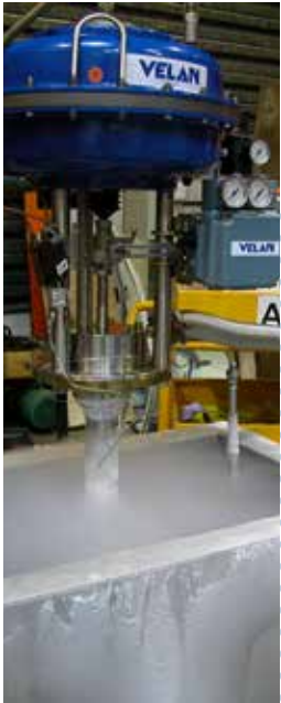
Cryogenic test in Liquid Nitrogen
