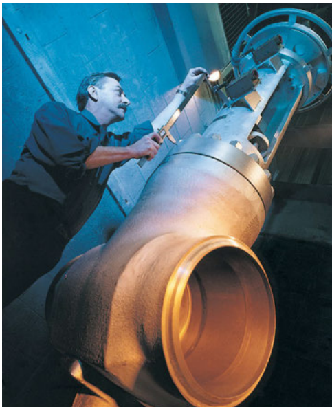
On-line statistical process control (SPC) is used on a y-pattern globe body after machining.
