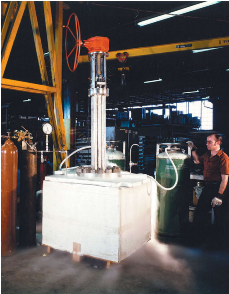
Velan employee Jack Kuhner performs cryogenic testing with liquid nitrogen on a Class 1500 steel gate valve. Jack went on to become one of Velan's first field sales technicians, traveling the world to work with customers.
