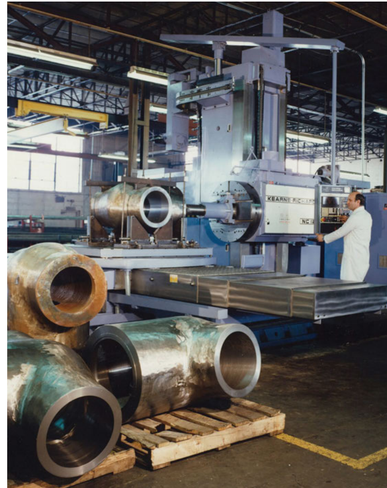
Machinery and equipment were specially engineered to meet the requirements of advanced large forged valve manufacturing. This included computer numerical control (CNC) horizontal and vertical boring mills with tool changers, numerical control (NC) lathes, and NC machining centers for valve and body parts. At the time, over 50 CNC machines were in operation in Velan's North American plants.
