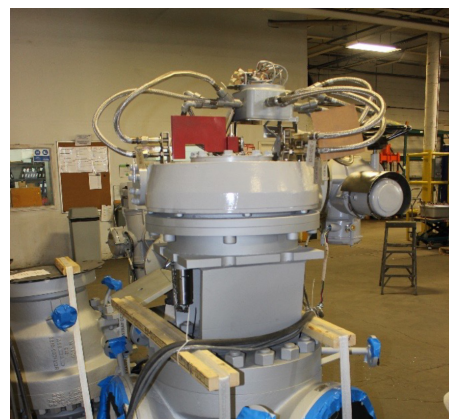
Typical external limit switch arrangement providing position indication (e.g., drum A, mid-point, drum B, bypass). Class 1, Div 1 or 2 or CENELEC explosive proof construction & Signal redundancy included. Signal available for local panel and/or remote DCS location.
