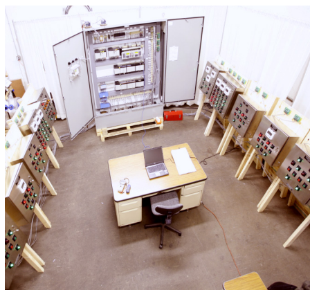
Velan PLC System featuring Fieldbus with diagnostic capabilities, control of interlock and permissives, HMI screen for system monitoring, DCS communication and handshaking, and an option for intrinsically safe signals.
