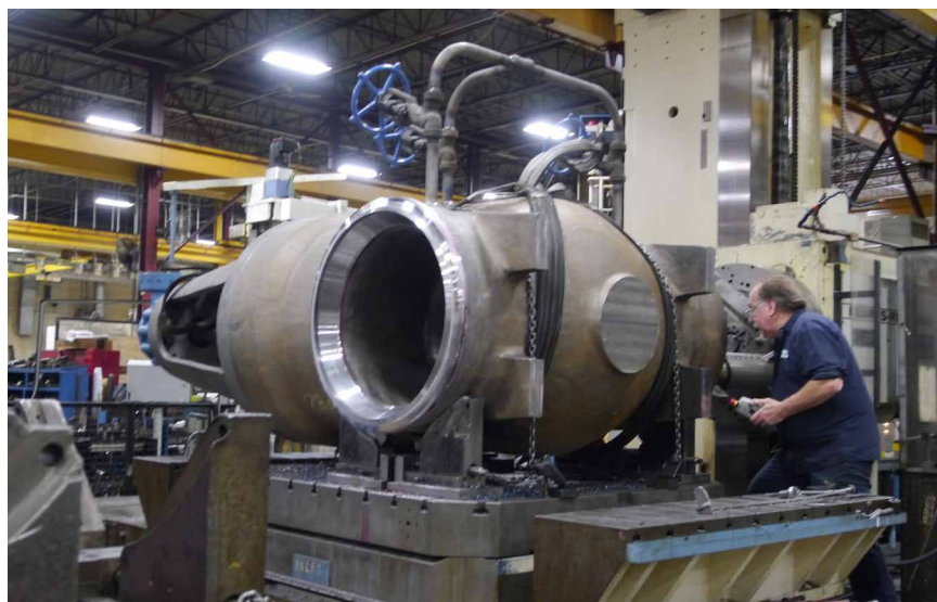
36" (914 mm) Class 900 carbon steel gate valve.
