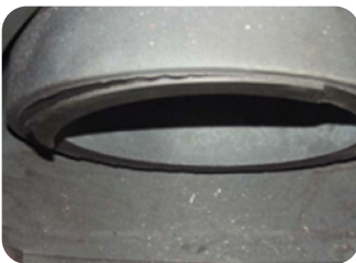
Stellite™ hardfacing delamination of a seat ring*
